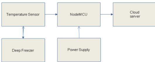
The PT100 Thermocouple is Industrial Temperature sensor we are using for this project the sensor is programmed in Node MCU to get the temperature of the deep freezer the data will store on cloud server to monitor w.r.t date and time as well as in the form of graph
